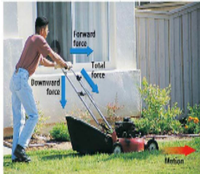
Figure 3 When you exert a force at an angle, only part of your force does work—the part that is in the same direction as the motion of the object. Compare the sizes of the total force and the forward force exerted on the mower.
